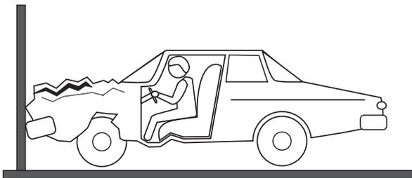
Within 1/10 of a second, the car has come to a stop, but the occupant continues to move forward.
